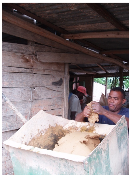
Figure 5 – Silver is mixed into the water to insure a homogenous mixture is attained
