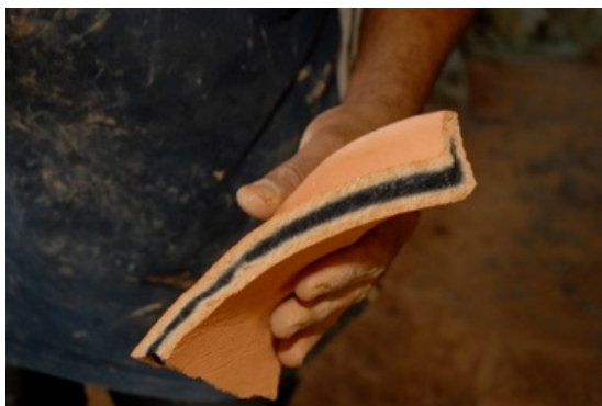
Figure 2 – Cutaway of filter showing charcoal integrated into the core
