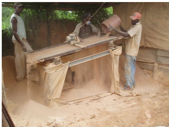
Figure 4 – Sifting materials through a fine mesh screen
